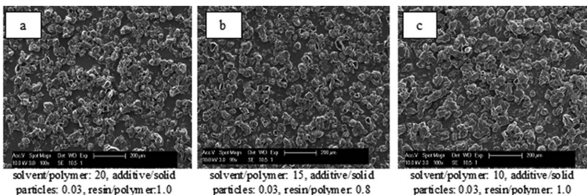
Figure 8. Effect of additive addition on distribution of resin particles ( \times 100 magnification).
